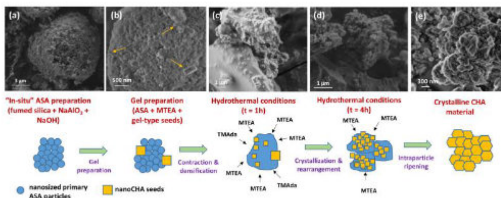
Figure 1. FESEM images of the solids achieved and proposed crystallization mechanism at different synthesis steps.
